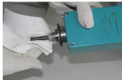
4. **Moisten the sensor with the phosphoric acid solution by slowly dripping 10 to 15 drops directly on the probe while rotating the unit. Drip enough of the solution onto the probe until the surface is completely covered.**
