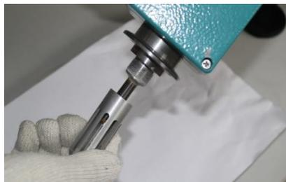
3. Apply distilled water on the sensor probe. Dry with a lint-free cloth (do not use paper towels). Handle the probe with care. Avoid excessive contact the surface of the probe.
