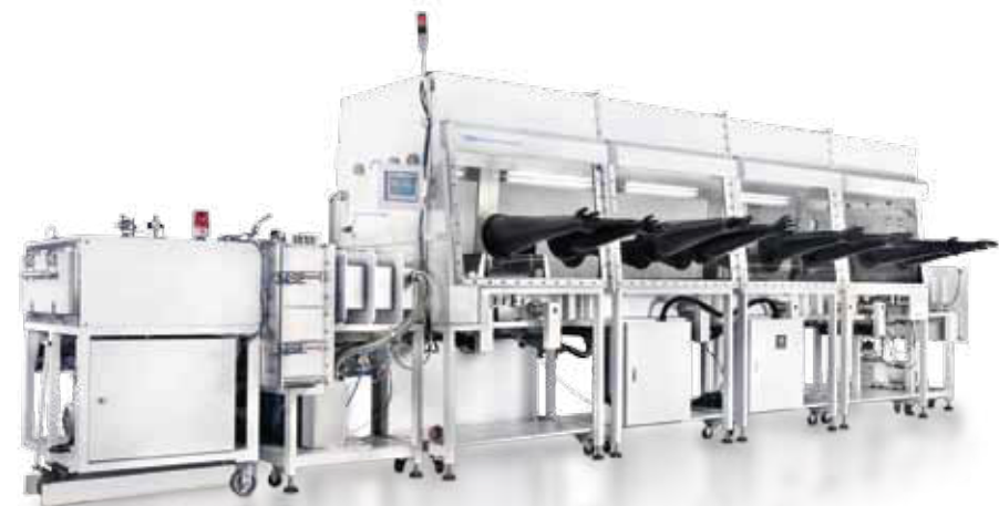
Circulation system (blower) Purification system (molecular sieve and copper-based catalyst) Renewable organic solvent absorber HF (hydrofluoric acid absorber)
