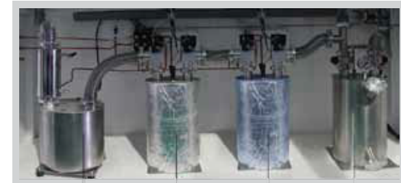
Circulation system (blower) Purification system (molecular sieve and copper-based catalyst) Renewable organic solvent absorber HF (hydrofluoric acid absorber)
